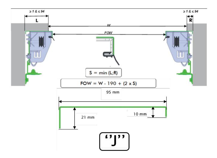
Optional – in case of the side room from 24 mm to 94 mm, it is possible to use vertical sealing with broken thermal bridge.
