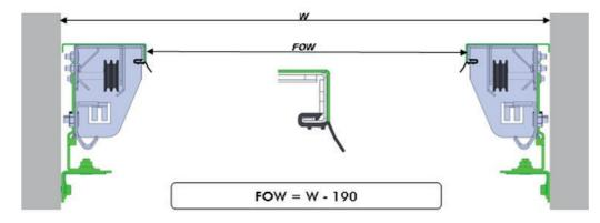
Standard – Vertical cover profile "J" with low sealing. Installation into opening.
