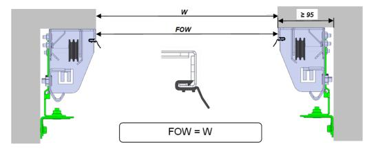
Optional – Vertical sealing with broken thermal bridge.
