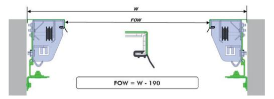
Optional – Vertical cover profile "L" with low sealing. Installation to match the façade of the house.
