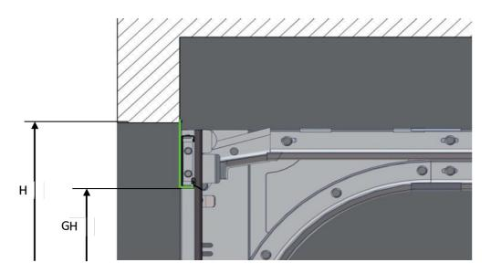
Option of installation of the horizontal cover "L" profile at: H - GH = 116 to 209 mm.
