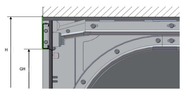
Option of installation of the horizontal cover "L" profile at: H - GH = 116 to 209 mm.
